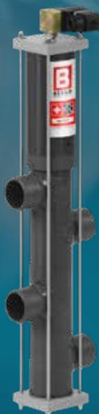
4-way valve, **including** 3/2 solenoid valve, 230 V, 1/4", with manual override. For switching the bypass to the solar system.
